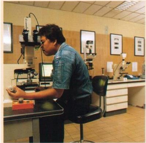
Metallographic examination using an optical light microscope
