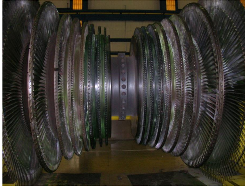
Low Pressure (LP) Turbine Rotor, 2 x 8 Stages Tandem
