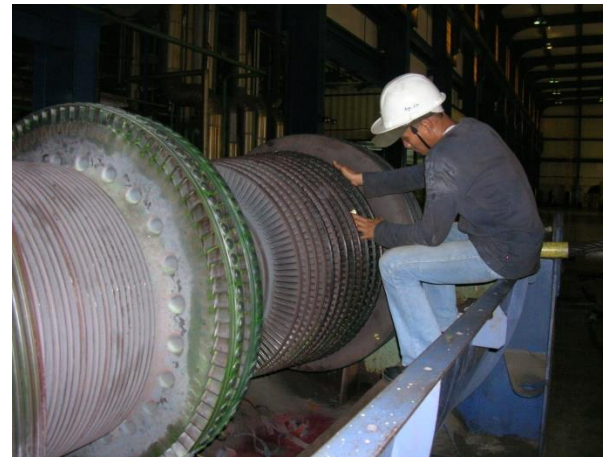
Intermediate Pressure (IP) Turbine Rotor (12 Stages) and High Pressure (HP) Turbine Rotor (12 Stages) with Curtis Turbine (2 Stages)
