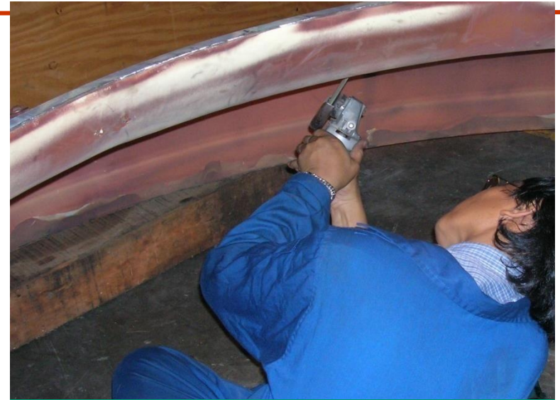
In-situ metallographic examination
