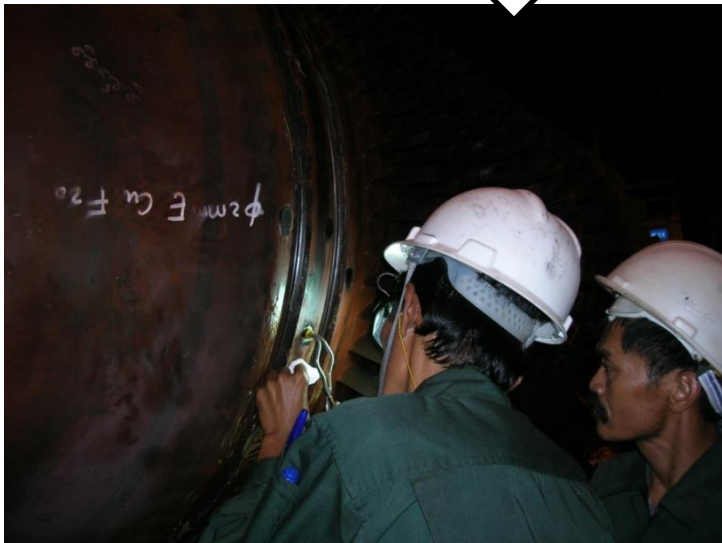
In-situ metallographic examination on gas turbine rotor
