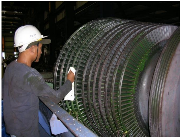
Intermediate Pressure (IP) Turbine Rotor (12 Stages) and High Pressure (HP) Turbine Rotor (12 Stages) with Curtis Turbine (2 Stages)
