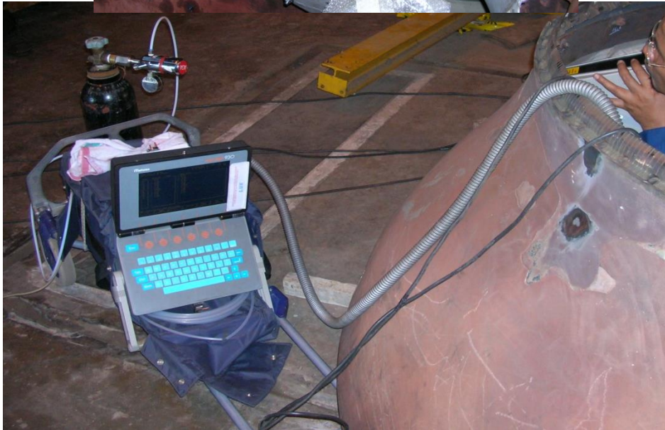
Chemical analysis by a portable Spark Emission Spectrometer
