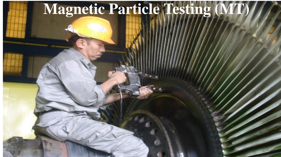
Magnetic Particle Inspection on stage 13 th (Christmas tree area)
