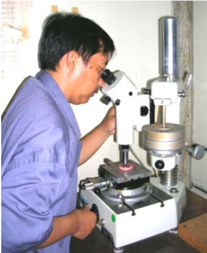
Vickers Hardness Method
