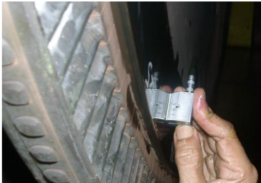
Scanning on straddle lip of disk
