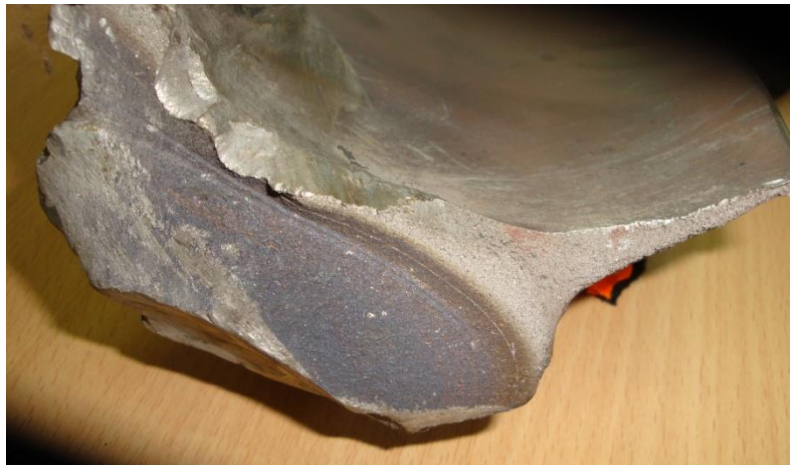
Fatigue Fracture Surface
