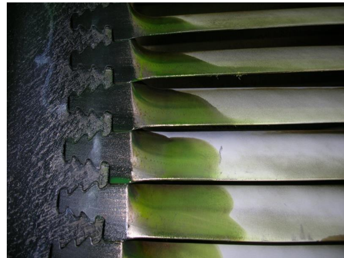
Christmas tree attachment of the blades last stage to the wheel disk rotor turbine
