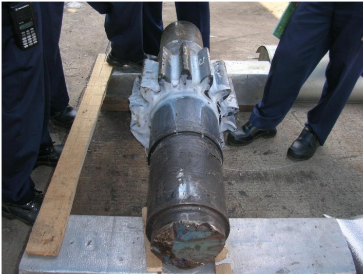
The fracture gear shaft that was photographed at the plant site.
