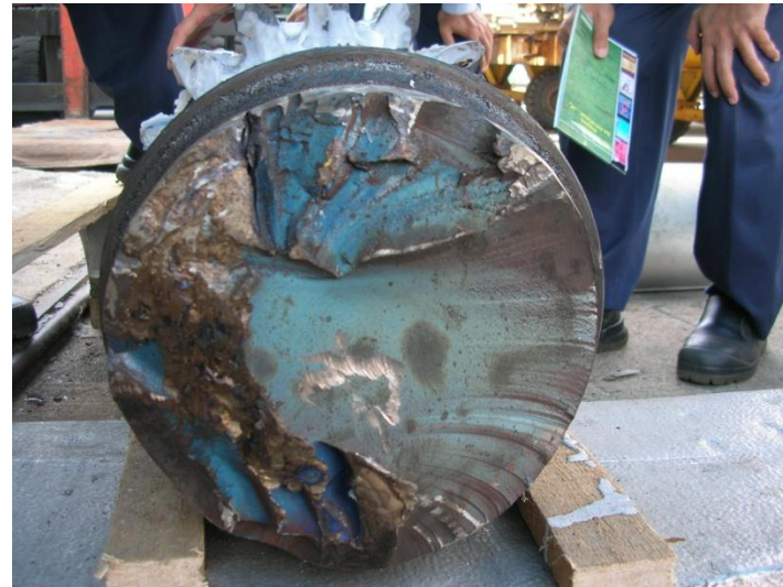
The fracture gear shaft that was photographed at the plant site.
