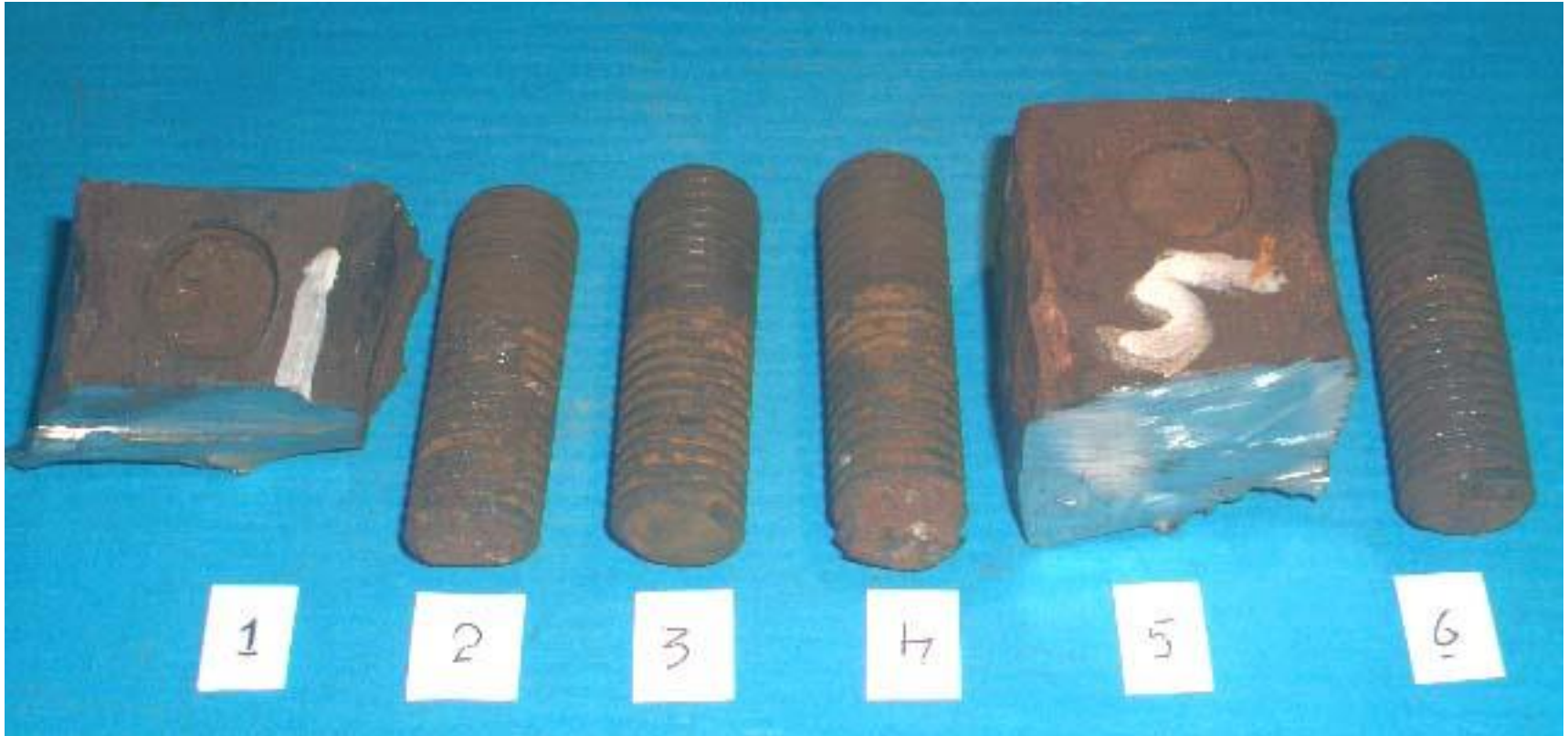
Close up view of the six broken stud bolts.
