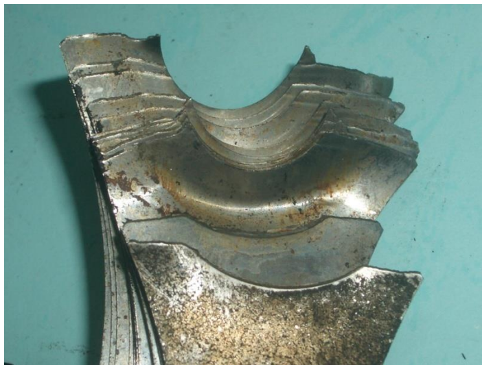
Macroscopic examination of the fracture surface of the broken disks (M Hub Ring A)
