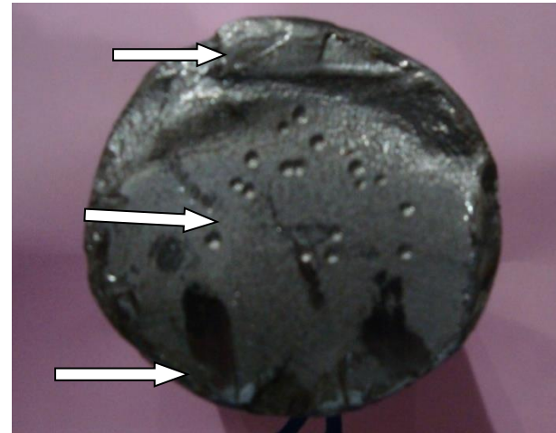
Fracture surfaces of the as received broken flight arms no. 1 to no. 4.
