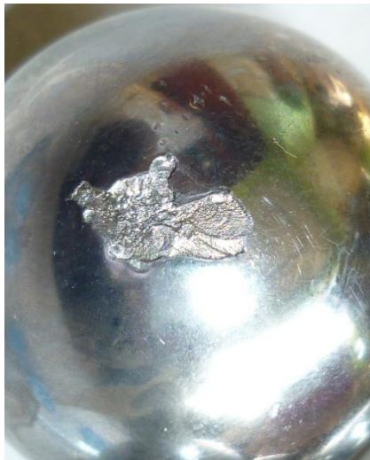
Close up view of surface damage formed on ball no. 1 of the damaged ball bearing
