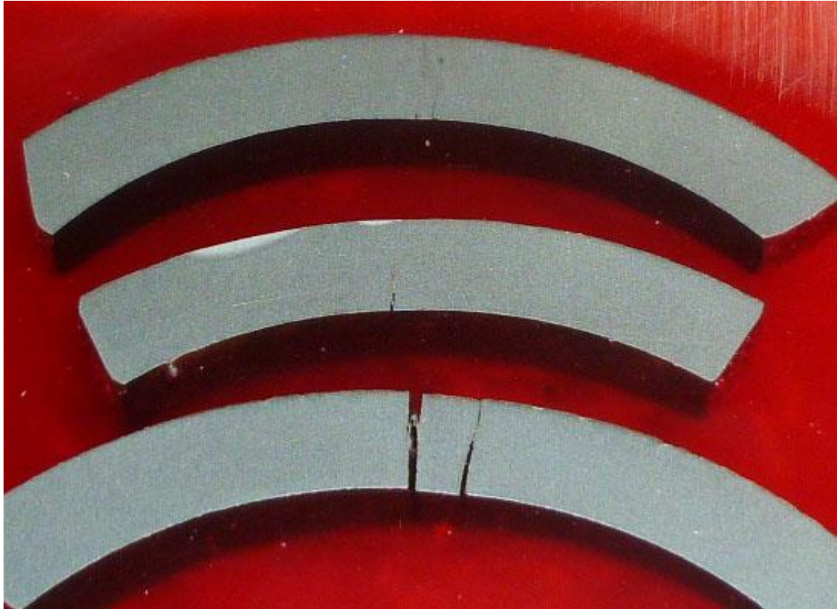
Specimens for metallographic examination of the fire side cracked tube
