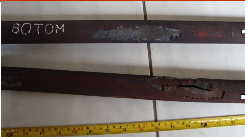
Tube burst due to long-term overheating
