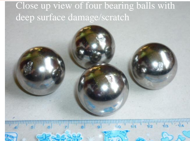
Formation of surface damage on a number of bearing balls
