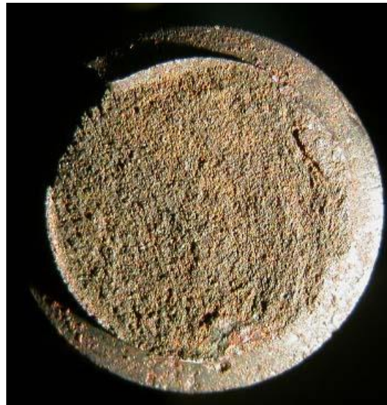
Fracture surfaces of the broken stud bolts showing chevrons or rays pattern.
