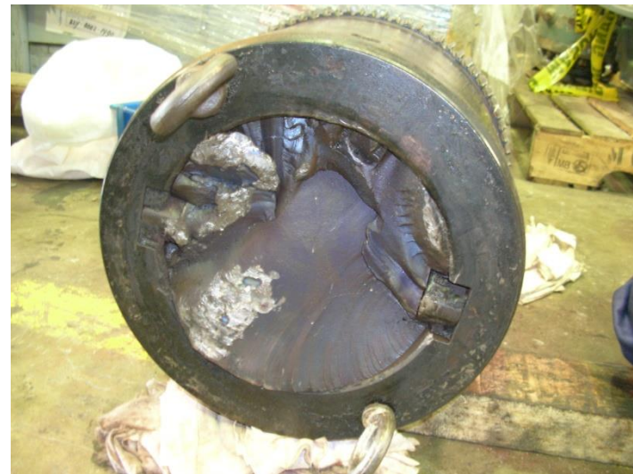
The fracture gear shaft that was photographed at the plant site.
