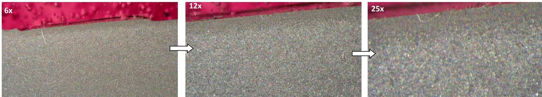
Macrostructures of the longitudinal section of the bent wheel stud of sample B at different locations and magnifications.
