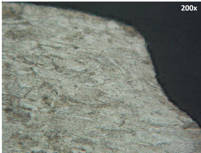
Microscopic examination of the cross section of the broken disk M Hub Ring A1
