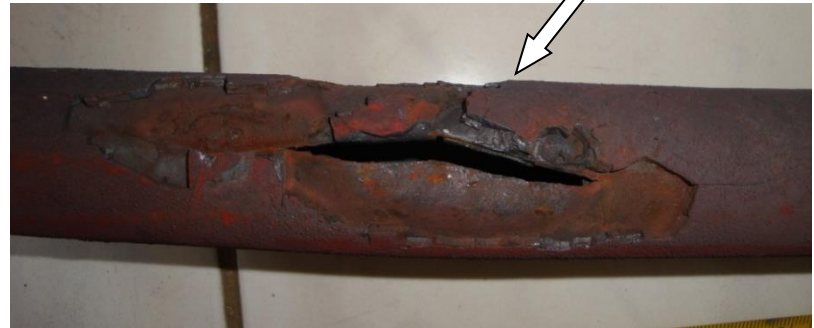
Tube burst due to long-term overheating
